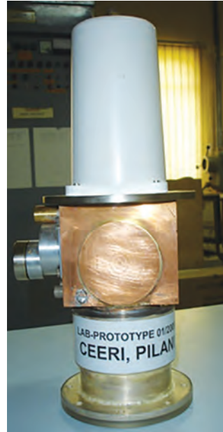
High-Power S-band, 2.6 MW Magnetron
