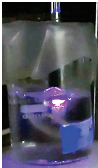
Cold atmospheric plasma single jet source for water treatment
