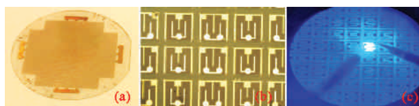
Photographs of fabricated blue LEDs on; (a) 2" wafer (b) enlarged microscopic image of LED, (c) blue light emission from fabricated blue LED
