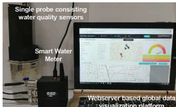
Developed technology for water quality and discharge monitoring
