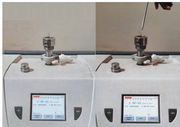
Helium leak test of header base
