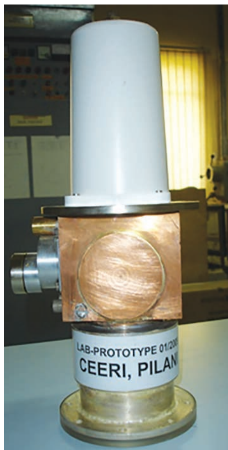
High-Power S-band, 2.6 MW, Magnetron
