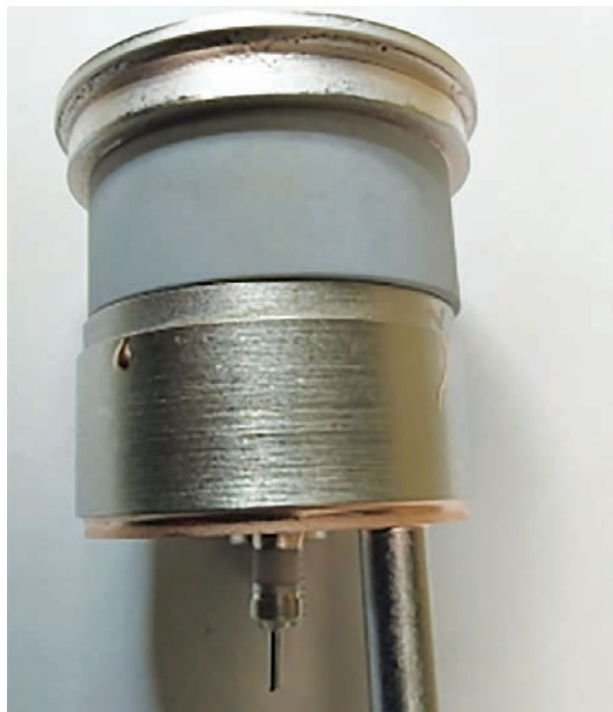
Developed sealed-off sheet electron beam source
