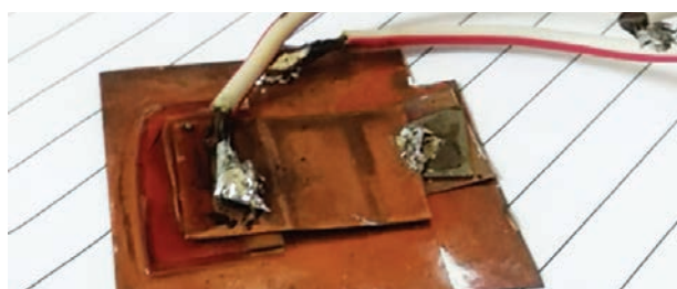
Packaging carried out in DRDO for high current testing
