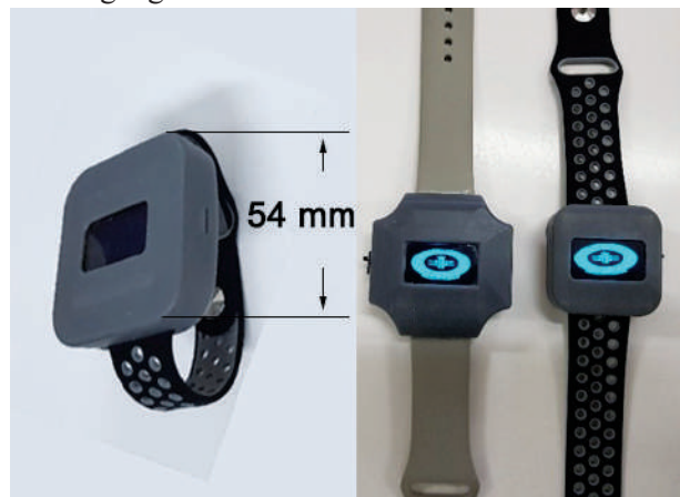
Realized multi-spectral PPG watches for HR, Blood oxygen saturation and HRV monitoring
