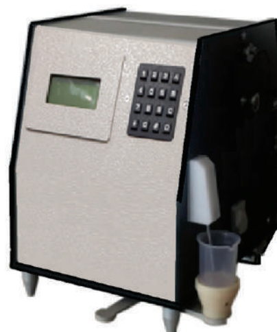
Milk supply chain adulteration monitoring system
