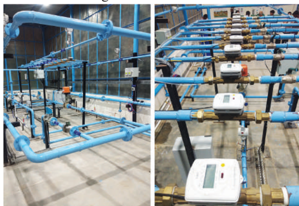
IoT based Smart Water Grid – Layer 1 & Layer 2
