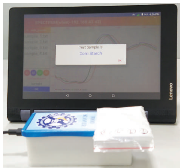
Portable version of the food scanner
