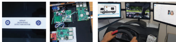
Prototype-I system for driver drowsiness detection integrating physiological (ECG) and behavioural measures on a resource constrained platform (RPI+NCS platform)
