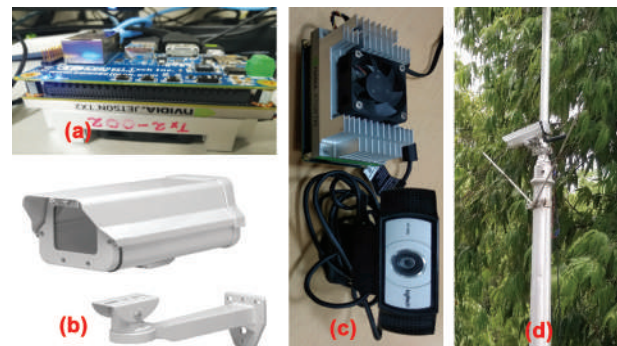
Components of Camera Module and Installation. (a) Connect Tech's Orbitty Carrier Board interfaced with NVIDIA Jetson TX2 (b) Camera Housing (c) Hardware module with Heat Sink and HD Camera (d) Installation of Camera module
