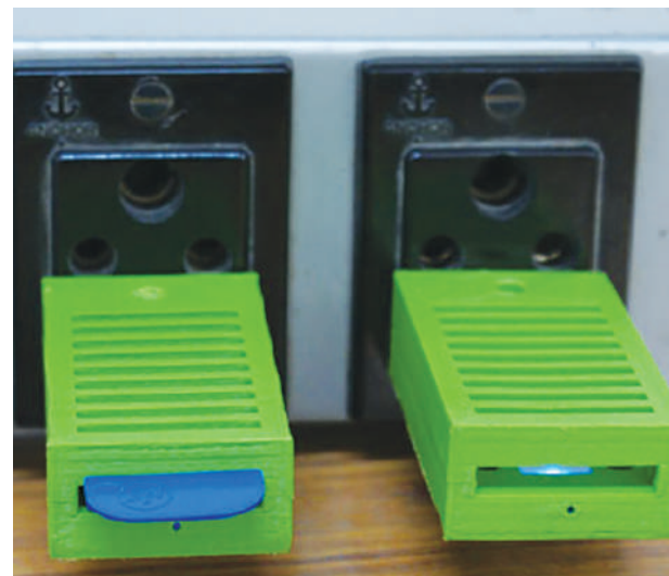
Thick-film hotplate integrated mosquito repellant unit
