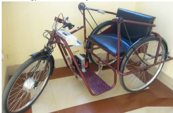
A prototype of developed e-trike for Divyangjan – the differently-abled person
