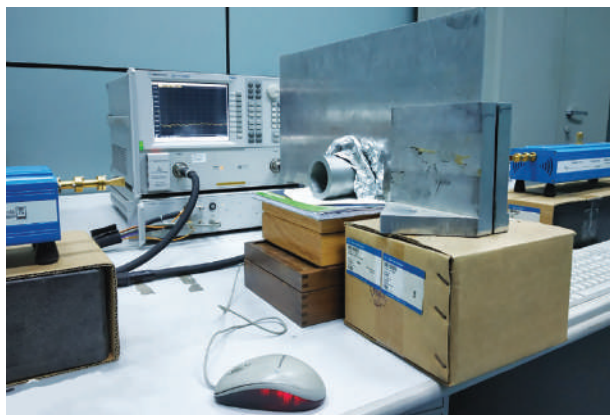
Test set-up and testing of the beam compression region
