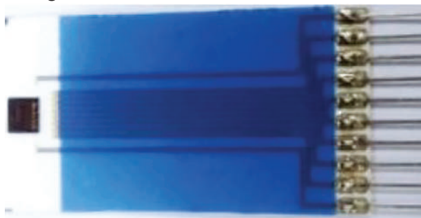
Packaged Si-FET device for biological applications
