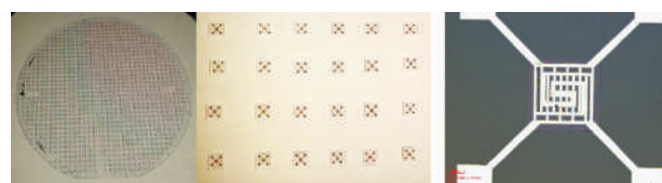
Optical images of processed glass wafer, micro gas sensor chips and micrograph of the micro gas sensor
