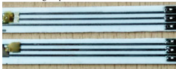
Packaged GaN HEMT devices for bio-sensing application
