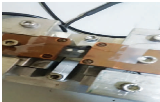
Graphene-polymer composite material, being characterized for strain sensing
