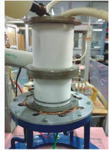
35 kV/3kA thyatron testing at BARC
