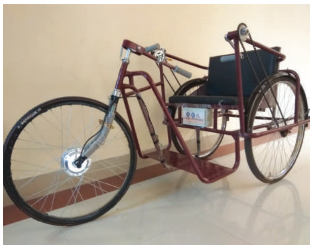
Implementation and testing of E-trike power assist
