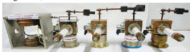
3 MW Magnetron prototypes with electromagnet
