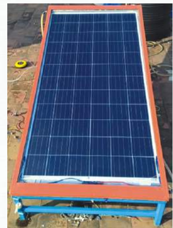
Photovoltaic-thermal (PVT) co-generation system
