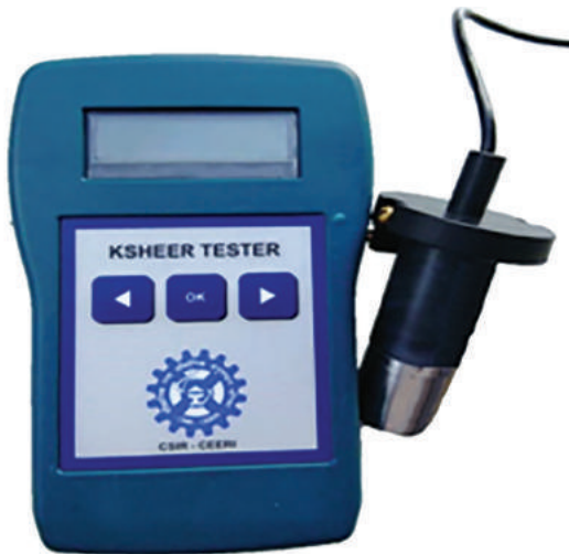
Ksheer tester (hand-held milk quality analyser)
