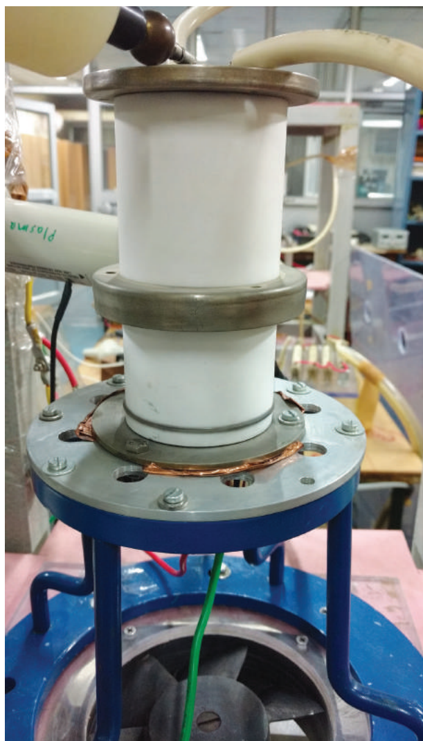
Developed third prototype of 35kV/3kA thyatron under testing at CSIR-CEERI
