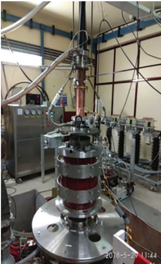
(b): Mounted gyrotron in the magnet system
