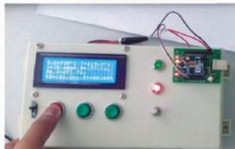
Gas detection system using IoT enabled packaged gas sensor
