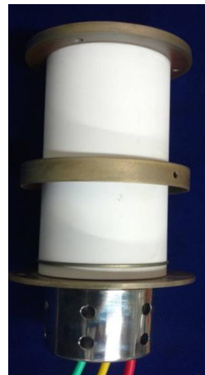
Figure 1: CSIR-CEERI developed 35kV/3kA Thyatron Plasma Switch
